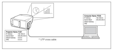
Connect the projector (PJ01) to the control computer (PC05) via the hub.
