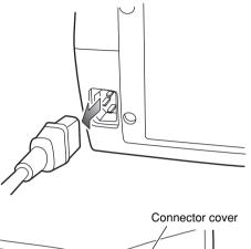
**2** Remove the connector cover and screw covers from the projector and insert plug on this product to the option connector.
