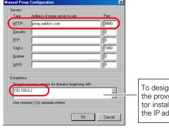
To designate proxy settings that will not use the proxy server when accessing the projector installed in the local area network, enter the IP address or domain name here.
