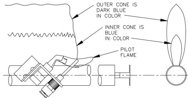
**Figure 9.1: Standing Pilot and Main Burner Flame**
