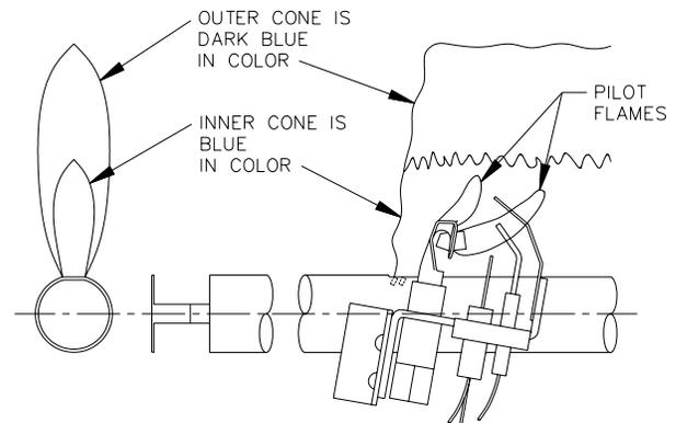
**Figure 9.2: Intermittent Pilot and Main Burner Flame**
