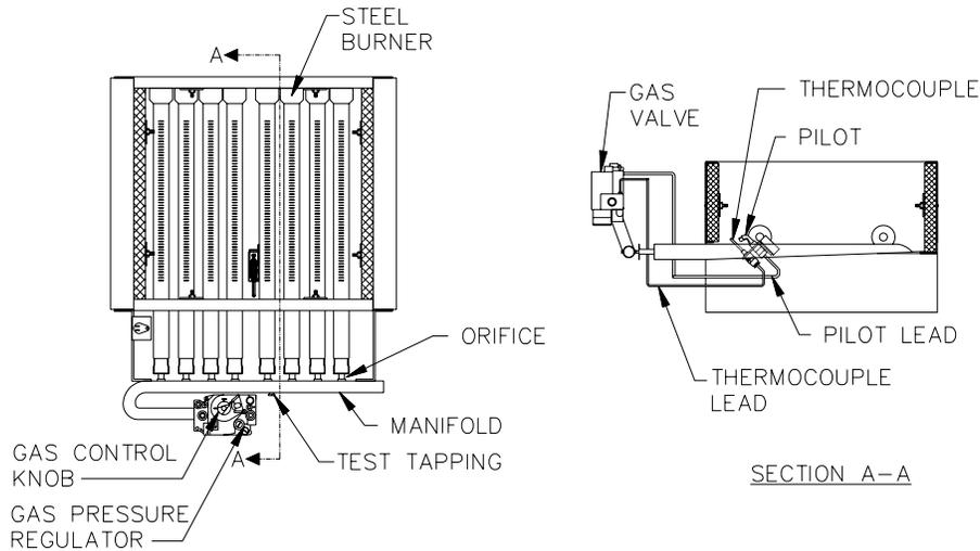
**Figure 7.1: Gas Valve, Manifold and Burner Assembly - Standing Pilot (Continuous Ignition)**
