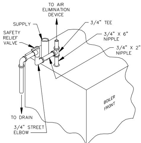
**Figure 3.4: Safety Relief Valve Hook-Up with Air Elimination**
