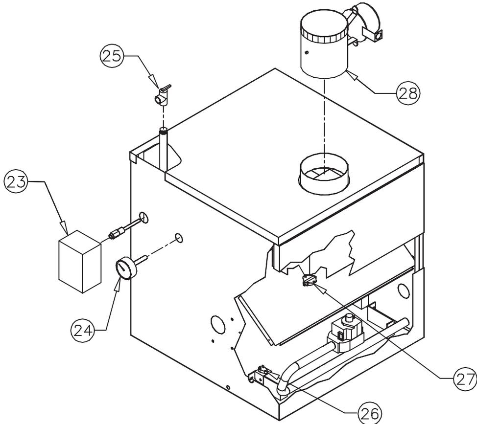
**Figure 11.6: Controls/Circulator/Vent Damper**
