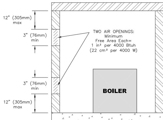
**Figure 1.3: Air Openings – All Air Directly from Outdoors**
