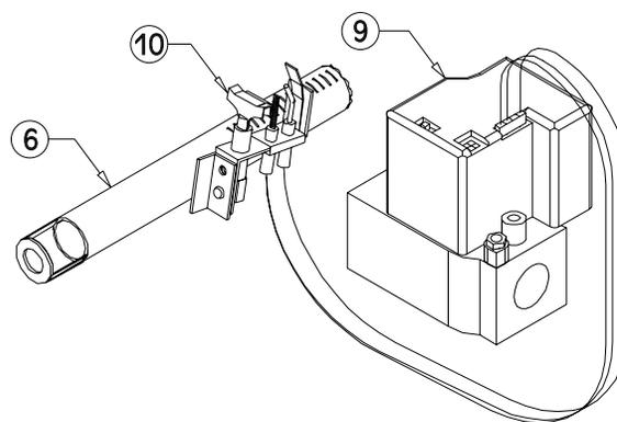
**Figure 11.3b: Gas Valve and Pilot – Intermittent Ignition**
