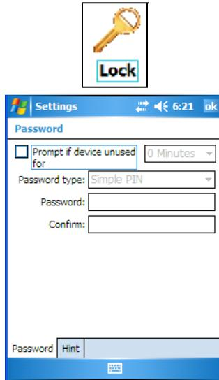
It is critical that you store your password in a safe place. If you forget it, a 'clean start' must be performed by certified Psion Teklogix personnel. A clean start returns the Ikôn to factory settings. Only the data stored in a CF or SD memory card are preserved.
