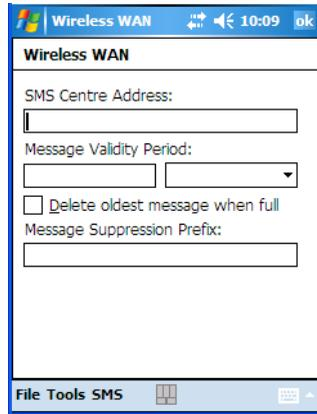
Tapping on *SMS Configuration* opens the SMS configuration dialog. The *SMS Centre Address* follows the same rules as the recipient's phone number in the *New* message dialog. The *Message Validity Period* parameter is sent to the SMS Centre with each message sent subsequently and instructs the SMS Centre on how long it should attempt to deliver the message to the recipient (the SMS Centre may impose an upper limit on the validity period regardless of the setting).
