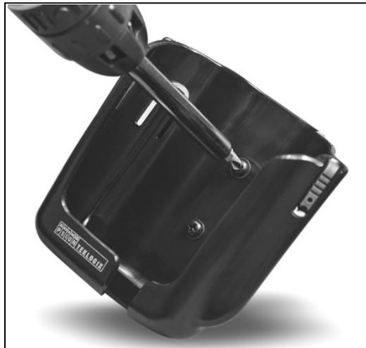
To accommodate the service loop of the power cable, leave a 10.2 cm (4 in.) clearance at the bottom of the vehicle cradle. Leave a 17.8 cm (7 in.) clearance at the top of the vehicle cradle to allow easy removal of the Ikôn. When selecting a mounting location, refer to the detailed assembly instructions that are packaged with the pedestal.
