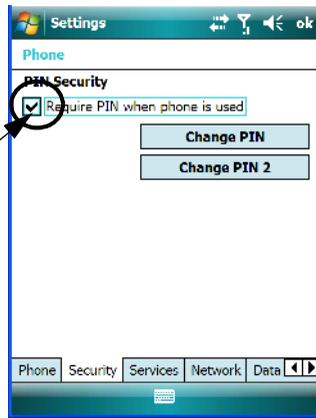
This option allows you to assign a *PIN* (Personal Identification Number) so that your PDA is protected from unauthorized use. Your SIM card manufacturer provides the default *PIN* which you can change in this field.
