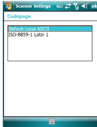
If you choose *Default Local ASCII*, the code page of the local OS is used. For example, if the local OS uses double-byte Chinese characters, choosing this option will filter data through the local ASCII of *that* OS and display it accurately, in this example, using double-byte characters.
