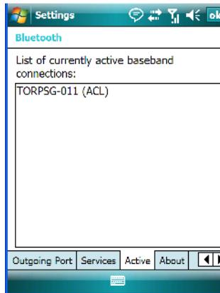
This tab displays the currently active *Bluetooth* connections, listing the device name(s). The type of link is also included with the device name(s). Keep in mind that the information listed in this tab is ‘view only’; it cannot be edited.
