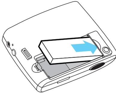
**2.** Align the battery so that the gold contacts on the battery match the gold contacts in the battery compartment.
