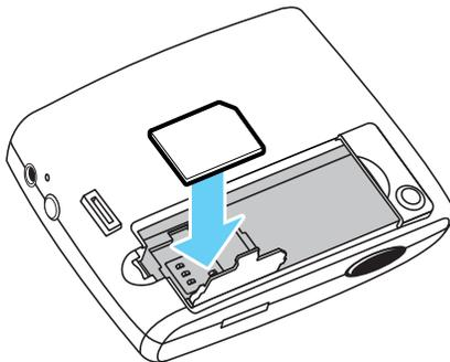
**1.** With the battery removed from the device, slide the small SIM gate in the direction of the arrow and lift it up.
