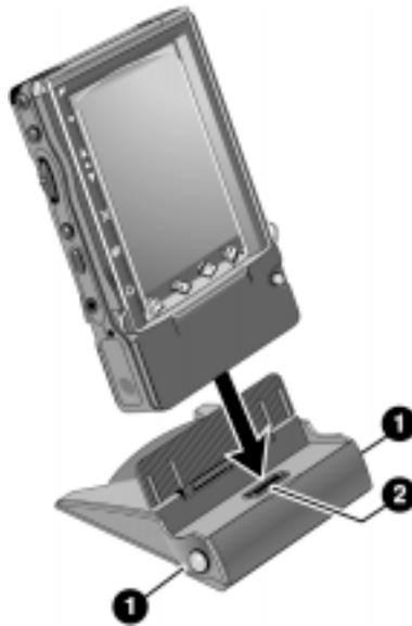
1. Release buttons—To release the HP Jornada from the cradle, press the buttons on both sides of the cradle.
