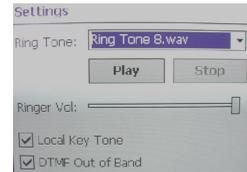
**To add a customized .wav file**, save the customized file in the Ring Tone wav field under the Program File\Inter-Tel\Model 8601\Ring.
