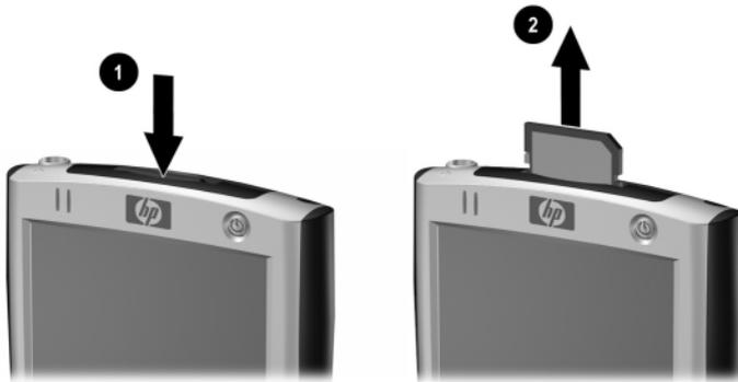
3. When the card disengages and pops up ❷, pull the card from the expansion slot.
