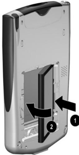
4. Replace the battery door by inserting it back into the tabs on the battery door area **1**, then close and latch it **2**.
