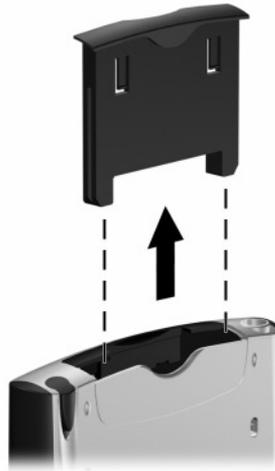
3. Insert the expansion card into the appropriate expansion slot and push the connection edge of the card firmly into the expansion slot.
