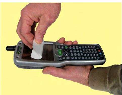
3. Align the exposed section of the protector with the bottom edge of the touch panel.
