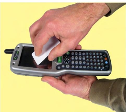
4. Apply the touch panel protector to your device by sliding the enclosed squeegee across the surface as you peel away the backing.
