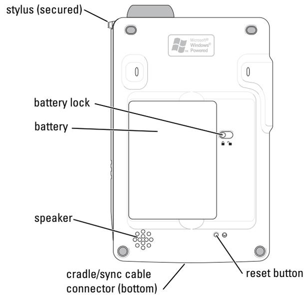
**BATTERY LOCK**—Use this switch to release and remove the main battery. See "Installing and Removing the Battery" on page 21.
