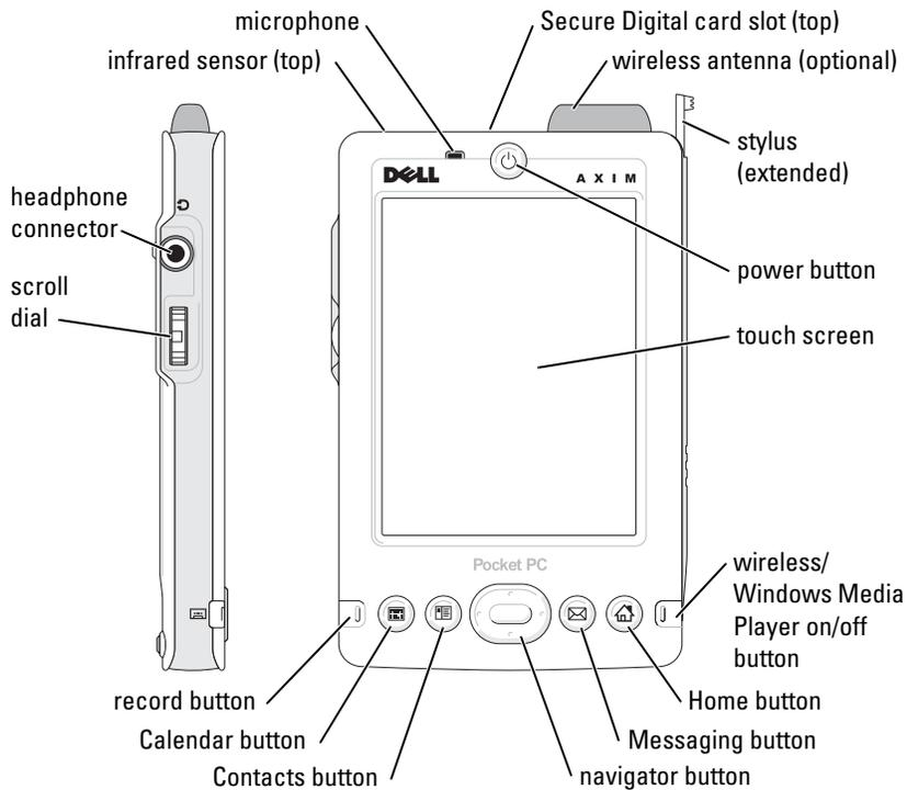
**INFRARED SENSOR**—The infrared sensor lets you transfer files from your device to another infrared-compatible device without using cable connections.
