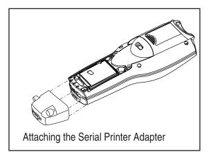
Once you have removed the strap studs, attach the adapter to the Falcon by sliding into place and tightening the thumbscrews on the adapter.
