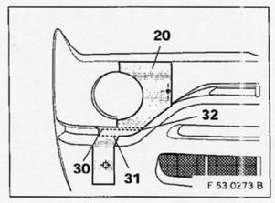
Remount the outer mouldings on the left and right. Remove the license plate and license plate amplifier.
