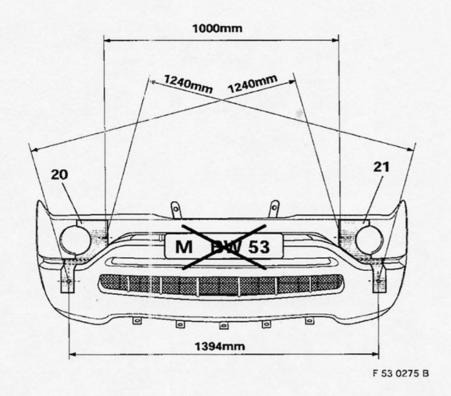
Check the proper positioning of the right-hand template (20) and the left-hand template (21) with the dimensions shown in the illustration.
