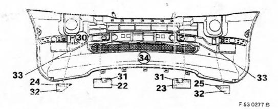
Glue the template for the upper left plastic spacer (22) and the template for the upper right plastic spacer (23) onto the plastic spacer (30) as illustrated.
