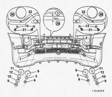
Insert the pre-assembled bar (1) into the holes of the bumper (30) front the front and push the two 60 mm dia. x 7 mm washers (6) onto the M6x70 set screws (2).
