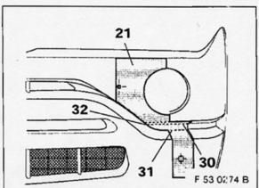
Cut out the left template (21). Start with line II (30) and line III (31) and put the template precisely at the left corner (32) of the depression of the cover and then stick the template on without making creases. (Line II (30) is the leader line).
