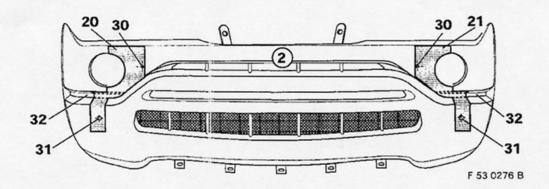
Drill the holes 8 mm dia. (30) and the holes 20 mm dia. (31) in the front apron (2) and deburr the holes.
