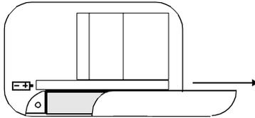
2. Remove the old battery, if necessary, and dispose of it properly.
