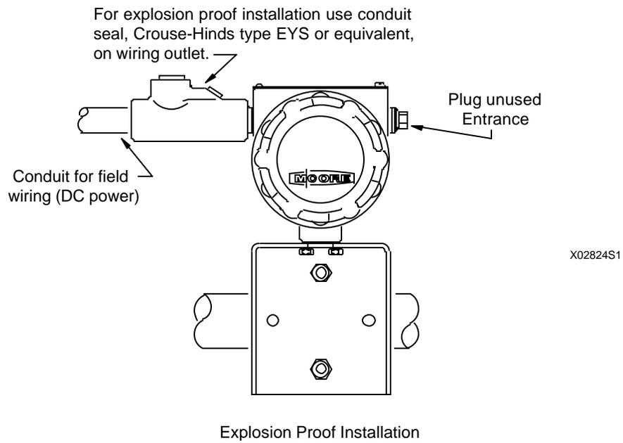
**FIGURE 4-11 Conduit Drain and Explosion Proof Installations**
