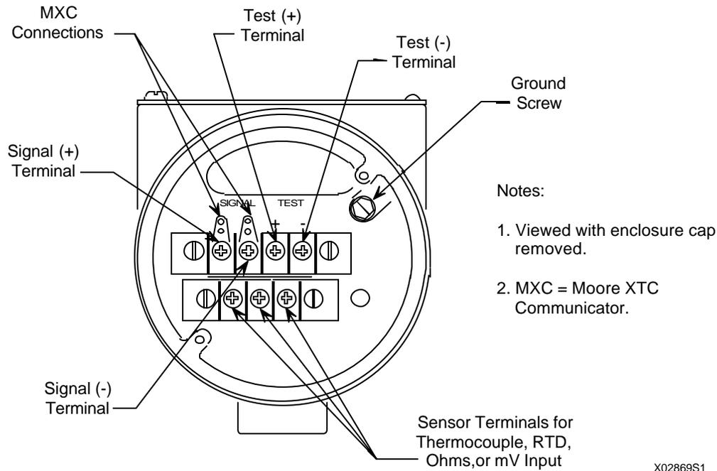
**FIGURE 4-12 Signal (Loop) , Sensor, MXC and Test Terminals**
