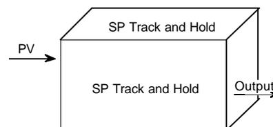
On power-up, the operating value in the function block is initialized to the Power-Up value. The Power-Up value can only be changed by editing the parameter in this function block with the MXC or by storing a new value via the pushbuttons of the XTC.
