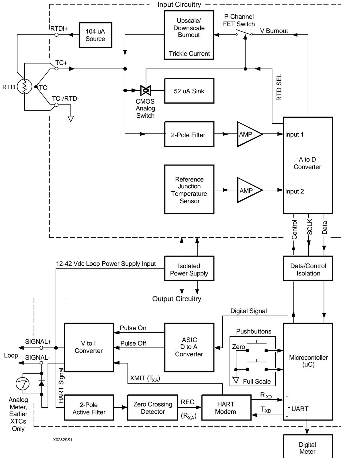
FIGURE 7-1 Model 344 Electronics Module Block Diagram
