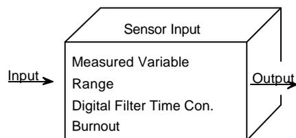
This function block allows the user to determine the range and the units in which the sensor will measure the sensor input. Range and span limits are dictated by a transmitter's sensor.
