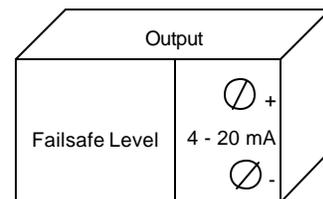
The failsafe level is the value to which the transmitter output will go if an error is detected while the transmitter is performing its self-diagnostic program. This value may be set at Lo ( $\leq 4$  mA), Hi ( $\geq 20$  mA), or at the last value the transmitter recorded before entering failsafe mode.
