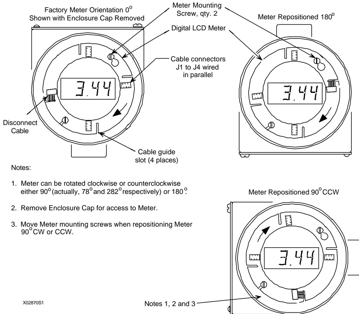
**FIGURE 4-10 Digital Meter Repositioning and Removal**
