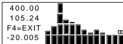
4) Press ENTER. The following are shown in the adjacent screen: Upper and Lower Range Values stored in the transmitter, the current transmitter reading and the thirteen sample trend.
