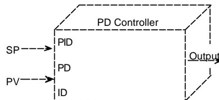
The PD controller is a proportional only controller with manual reset which can be selected as tracking or non-tracking.
