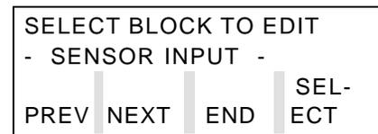
All MXC screens have a similar layout. As shown here, most configuration screens use the top two lines to describe the current screen, and the lower two lines to show the selections available from this screen. Selections are entered by pressing keys on the MXC keypad. Some on-line variable and trend screens are slightly different from that shown here, but they will always have a selection to access the next screen.
