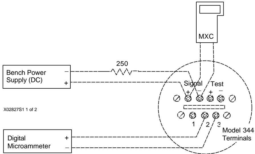
**FIGURE 6-3 RTD/Ohm Current Source Calibration Set Up**
