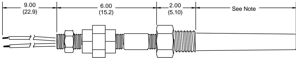
Thermocouple Thermowell Assembly
