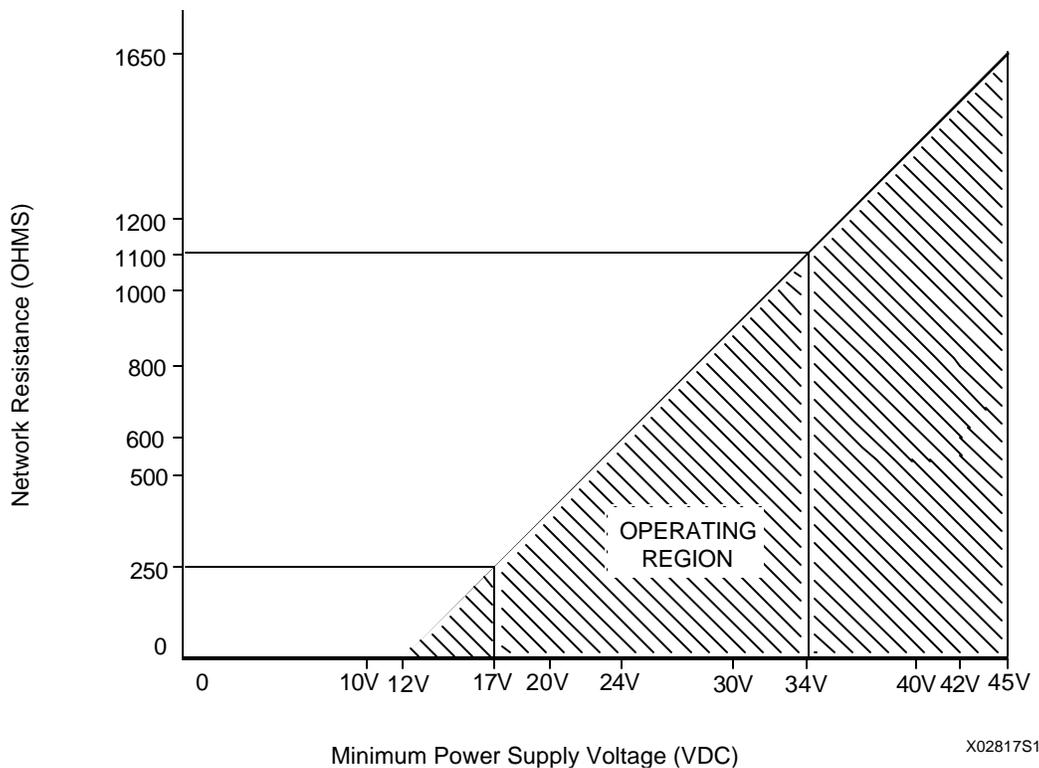
**FIGURE 4-4 Supply Voltage Versus Network Resistance**
