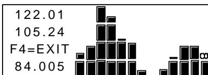
The MXC will display the trended variable within the zoom range chosen (i.e. zoom range = 10% of the transmitter range, centered on the zoom value entered) on the screen. The screen will show:
