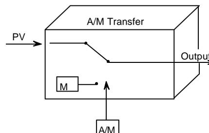
is in MANUAL, the output is the manual (M) value (-1.0 to 110%). The manual value can be adjusted with the pushbuttons of the XTC or from the CHANGE VALVE key of the MXC. When the manual (M) value is not the function block output, it will track the output value of the controller function block.
