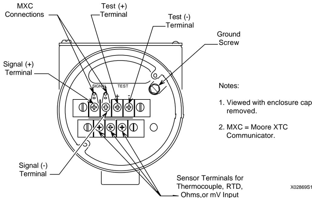
**FIGURE 1-2 Terminal Connections**
