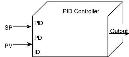
The PID controller is a reset type controller which uses external feedback to establish the integral action. The function block will force the output to track the feedback when the controller is in manual. If the derivative time TD is set to 0.00, the derivative section is eliminated.
