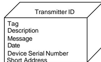
The Transmitter ID block contains ASCII strings that can be entered to aid in record keeping and identification of the transmitter. These ASCII strings include an 8-character Tag, a 16-character Descriptor, and a 32-character Message. In addition, a date code and an 8-digit Device Serial Number that can be used to identify the transmitter can be entered.
