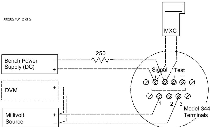
**FIGURE 6-4 TC/mV Input Accuracy Check and Calibration Set Up**
