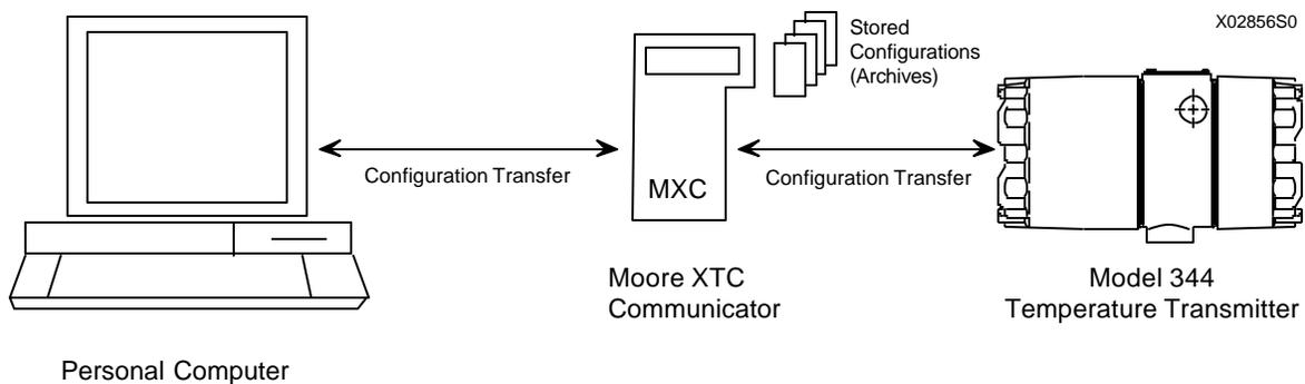
The MXC and the field instruments with which it communicates use the HART protocol for remote communications. HART uses Frequency Shift Keying (Bell 202 standard) to superimpose digital signaling on the standard 4-20 mA analog signal. Since there is no net energy change, the analog signal will not be disturbed and loop integrity is maintained.
