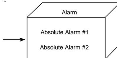
This function block includes 2 absolute alarms. The action of these alarms can be selected as HI or LO. The setpoint for the alarms is entered in the units selected in the operator display block.
