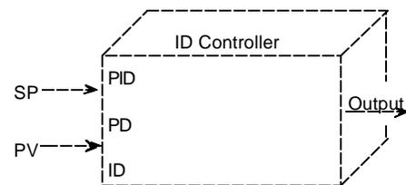
The ID controller is an integral only controller which uses external feedback to establish integral action.
