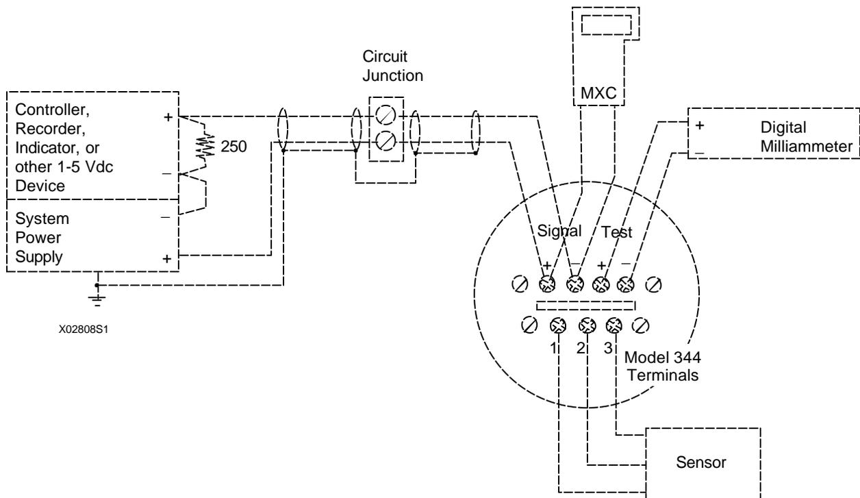
FIGURE 6-2 Field Calibration Connections
