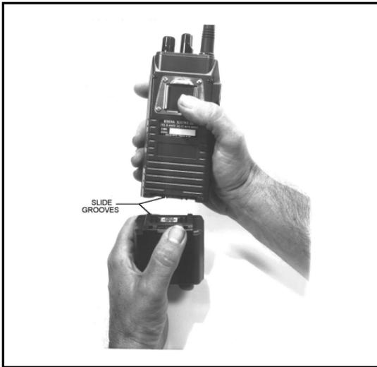
*Figure 8 - Installing the Battery Pack*
