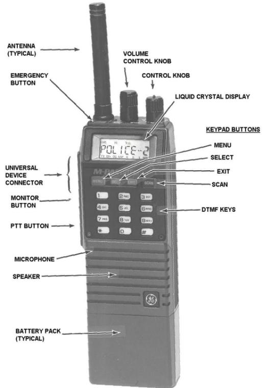
Figure 5 - M-PA System Model Radio
