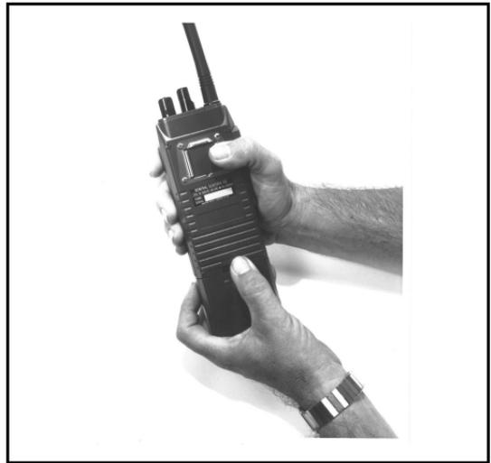
*Figure 9 - Removing the Battery Pack*
