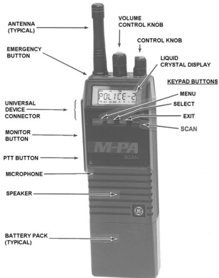
Figure 3 - M-PA Scan Model Radio
