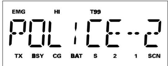
Figure 7 - Liquid Crystal Display
