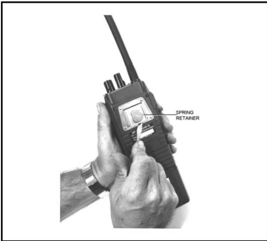
Figure 10 - Swivel Mount Removal and Replacement
