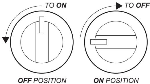
Fig. 4 Burner Control
