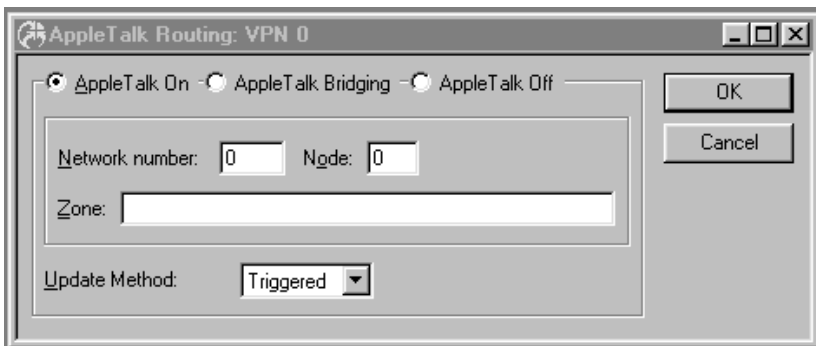
AppleTalk Routing: VPN Configuration Dialog Box
