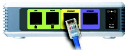
Figure 4-3: Connect a PC
