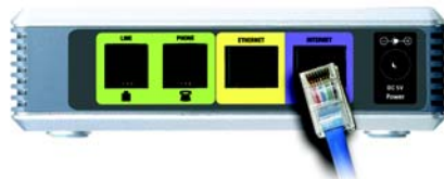
Figure 4-4: Connect to the Modem
