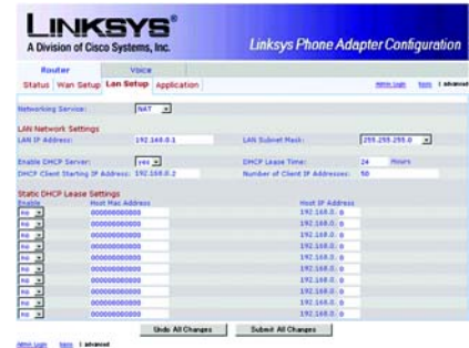
Figure 6-6: Router - LAN Setup Screen
