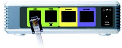
Figure 4-1: Connect to the Telephone Wall Jack
