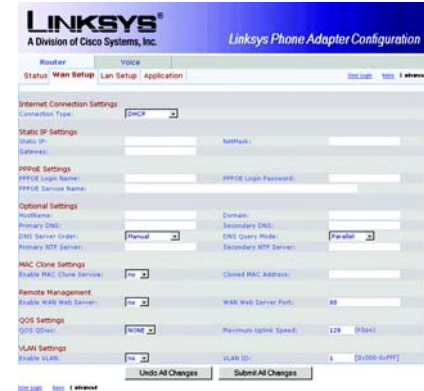
Figure 4-7: Router - WAN Setup Screen
