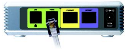
Figure 4-2: Connect a Telephone
