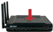
**AOSS** (AirStation One-Touch Secure System) is a simple system for configuring your wireless network securely. If your router and your client device are installed and both support AOSS, then making a secure wireless connection between them is simple.
