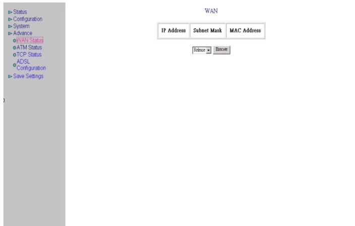
Each VC setting you enabled in the **WAN Configuration** section except that uses the PPP encapsulation will be displayed in this table.
