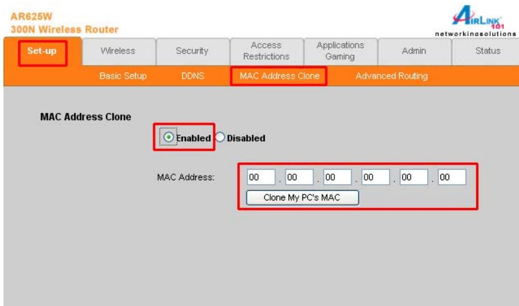
The screenshot shows the 'MAC Address Clone' configuration page. The 'Enabled' radio button is selected and highlighted with a red box. Below it, the 'MAC Address' field is set to '00 . 00 . 00 . 00 . 00 . 00' and is also highlighted with a red box. A 'Clone My PC's MAC' button is located below the MAC address field.
