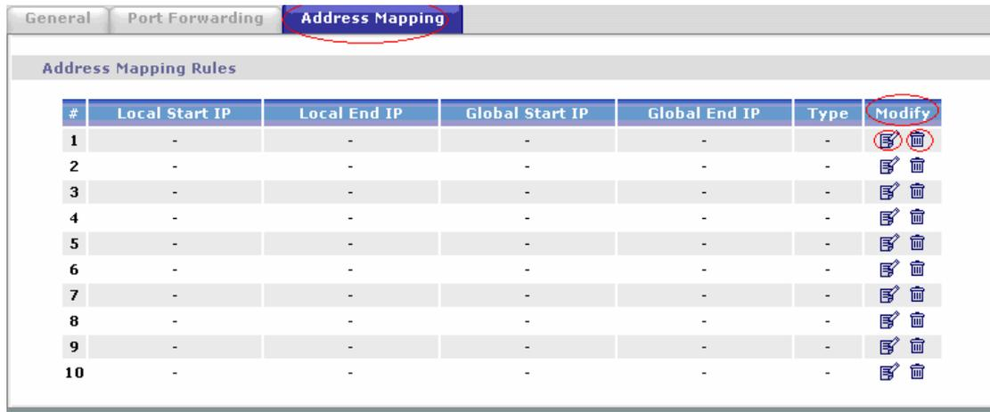
This menu is for Address Mapping Set #1, you can edit 10 Address Mapping Rules for Set #1. You can edit or remove a rule by clicking the two buttons on the rule table.
