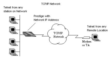
Figure 13-1 Telnet Configuration on a TCP/IP Network
