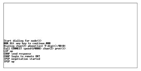
Figure 14-7 Trace Display for a Successful IPCP Connection via Manual Call Below is an example of a failed Trace Display for a Successful IPCP Connection via Manual Call.
