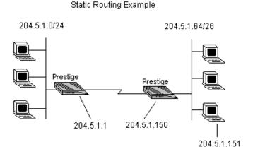
Figure 7-4 Static Routing Example
