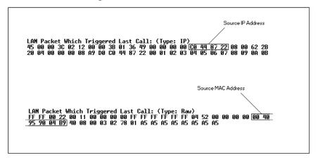
Figure 14-3 LAN Packet Which Triggered Last Call
