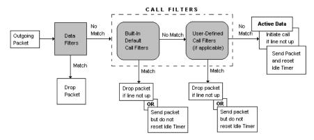
Figure 10-1 Outgoing packet filtering Process
