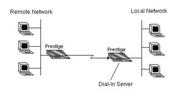
Figure 6-2 Example of a Dial-In Server Application
