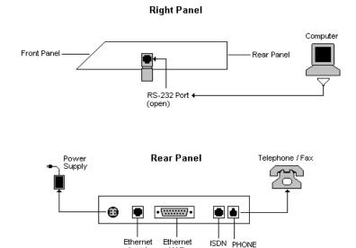
Figure 3-1 Rear Panel Diagram
