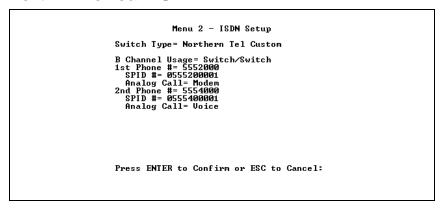
Figure 3-7 Menu 2 - ISDN Setup for North America
