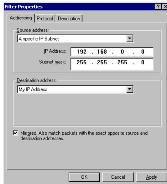
**Figure 71: Filter Properties: Addressing**
