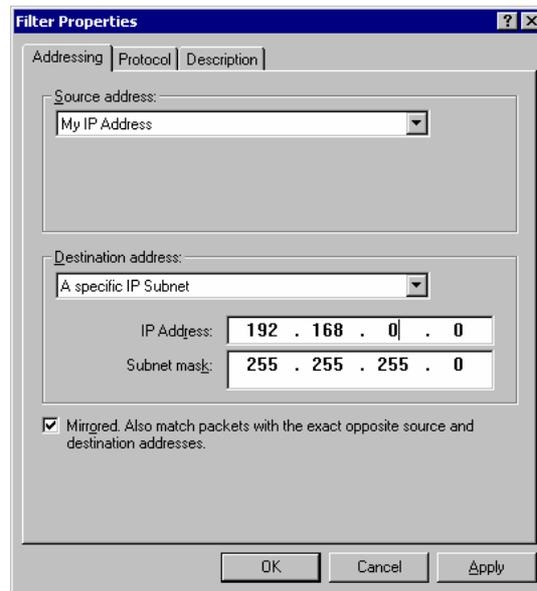
**Figure 61: Filter Properties: Addressing**
