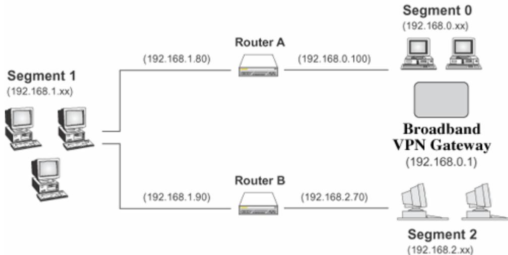
Figure 117: Routing Example
