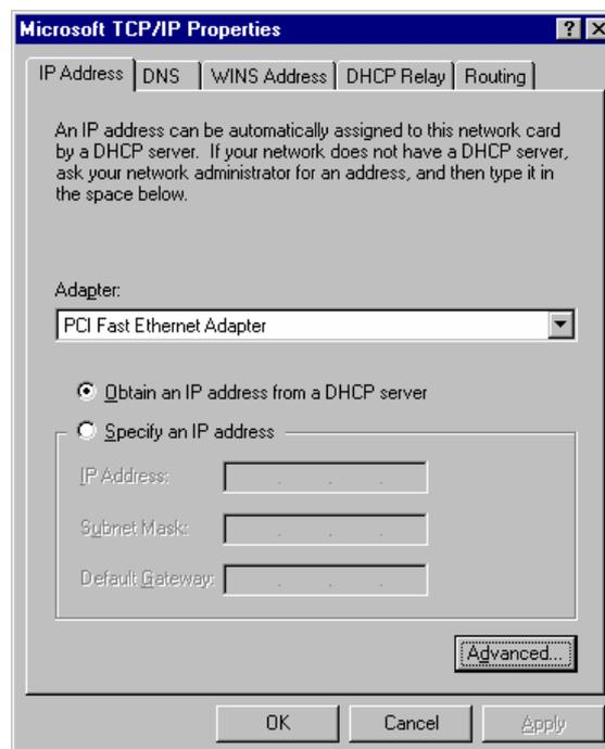
**Figure 13: Windows NT4.0 - IP Address**
