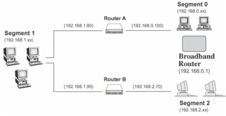
**Figure 52: Routing Example**
