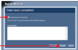
9. Verify that the test has completed successfully. Check that the ADSL and Internet LEDs are lit. Then click **Close**.
