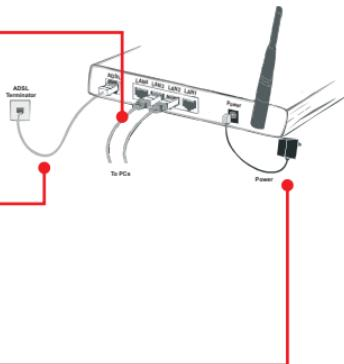
2. Connect one end of the RJ-11 cable to the TEW-436BRM's ADSL port. Connect the other end of the cable to the phone jack.
