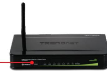
3. Connect the AC Power Adapter to the TEW-436BRM and then to a power outlet.
