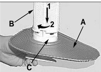
Reassemble the filter parts (as shown in the figure) and reinsert the whole assembly into the dishwasher. Position it into its housing and press downwards. The dishwasher is not to be used without filters. Improper replacement of the filters may reduce the efficiency of the wash and even damage your dishwasher.
