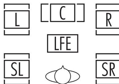
These indicators are the L/C/R/LFE/SL/SR letters that are inside the center boxes of the **Speaker/Channel Input Indicators 14** in the front panel **Main Information Display 23**.
