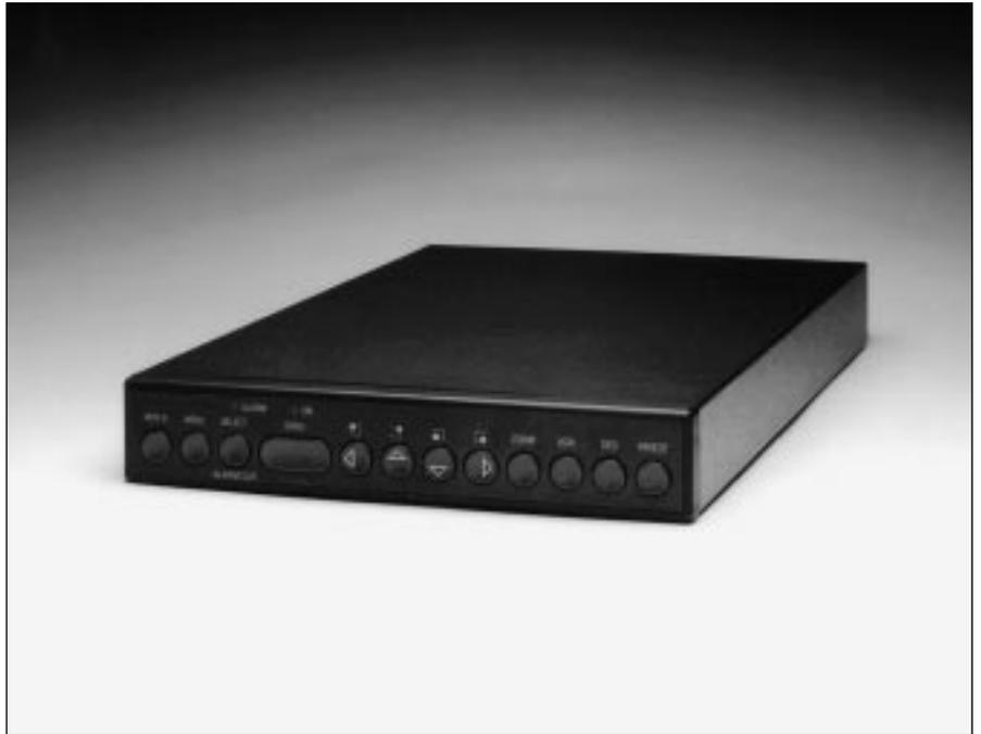
The TC8278 Series video processors digitally capture the full video from up to eight sources, display them selectively full screen, or reduces these images to quarter-screen size, and combines them to provide a two page quad display. The TC8278 Series will accept monochrome and/or color inputs and provide monochrome and/or color display capabilities in the full screen and quad modes.
