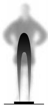
Tanita's patented "foot-pad" design sends a safe, low-level electrical signal through the body to determine its composition.
