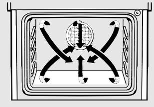
When you set the oven for CircuWave, a convection fan circulates the hot oven air over and around the food.
