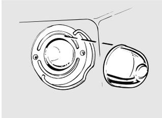
**CAUTION:** Before replacing your oven light bulb, turn the oven light off and disconnect the electrical power to the range at the main fuse or circuit breaker panel.
