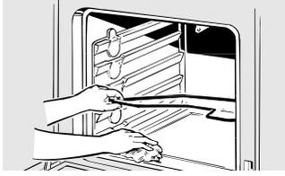
*Do not clean the bake element or the broil element. Any soil will burn off when the elements are heated.*
