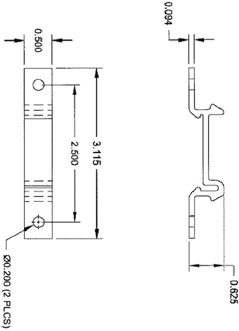
Figure 3: Mounting Clip Dimensions (units are inches)
