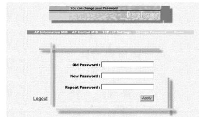
In the change password screen you may change the password on the access point. As password is required to configure the SMC2652W Access point. We suggest changing your password from the default to ensure network security.
