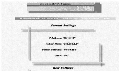
The TCP/IP settings page allows you to view and change the network settings on the access point.
