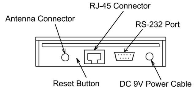
3. Connect the Ethernet cable - The SC2652W can be wired to a 10Base-T Ethernet network with a network device such as a hub or switch. Connect into the RJ45 connector socket on the back panel with category 3, 4 or 5 UTP Ethernet cable and an RJ45 connector.
