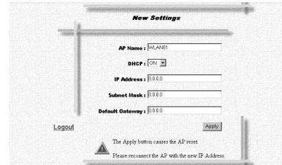
With DHCP “ON”, the IP address and subnet are set automatically. If you want to set these yourself, enter a new IP address and subnet mask in the “New settings” section of the “TCP/IP settings” screen, then click on “Apply”.
