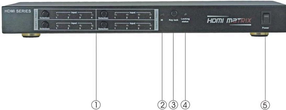
1. Output selection and indicator of input for output port 1 to 4.
