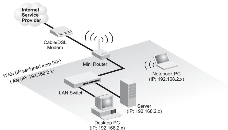
The private local network, connected to the LAN port or wireless interface, provides a Dynamic Host Configuration Protocol (DHCP) server for allocating IP addresses to local PCs and wireless clients, and Network Address Translation (NAT) for mapping the multiple "internal" IP addresses to one "external" IP address.
