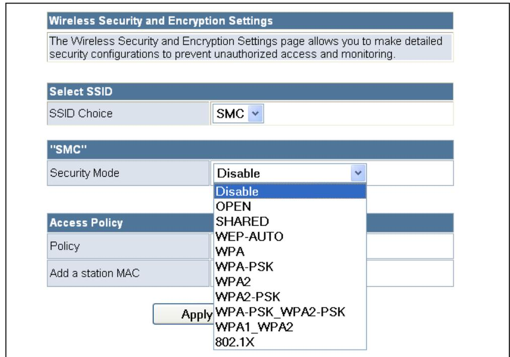
The supported security mechanisms and their configuration parameters are described in the following sections:
