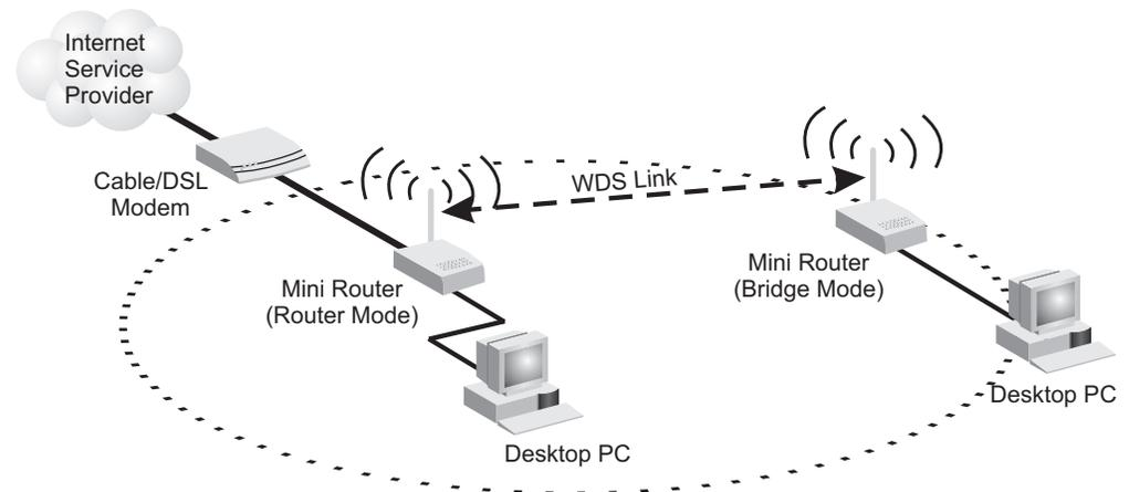
**Figure 8: Operating as a Wireless Repeater**
