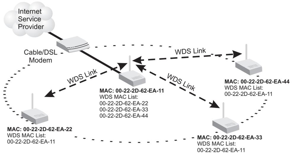
**Figure 47: WDS Configuration Example**
