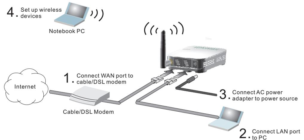
To connect the Mini Broadband Router in Router Mode for use as an Internet gateway, follow these steps:
