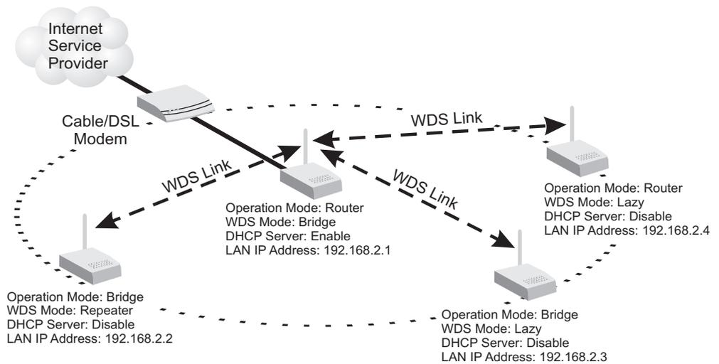
A WDS link between two units can be configured in any of the following Operation Mode combinations:
