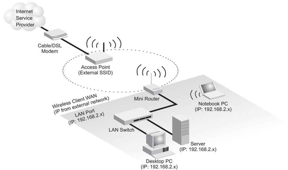
The Mini Broadband Router has two basic operating modes that can be set through the web-based management interface. For information on setting the mode suitable for your network environment, see [“Operation Mode” on page 50](#).
