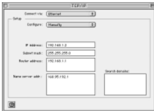
**Figure 25. Manual Configuration of IP Addresses**
