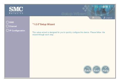
Service Set ID – Enter the service set identifier in the SSID box which all wireless clients must use to associate with the access point. The SSID is case sensitive and can consist of up to 32 alphanumeric characters. (Default: SMC)
