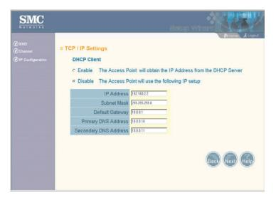
*DHCP Client* – With DHCP Client enabled, the IP address, subnet mask and default gateway can be dynamically
