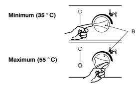
Adjustment of the DHW temperature is completely separate from that of the CH circuit.
