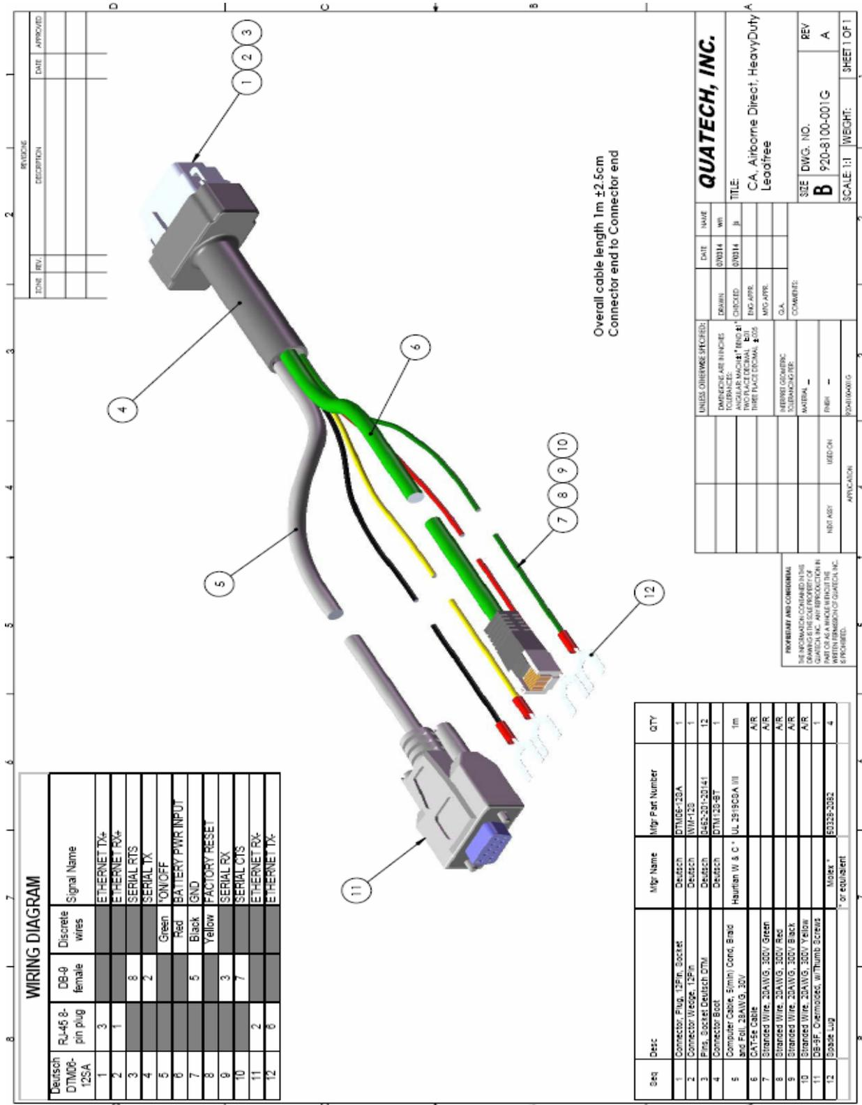
Figure 6. AirborneDirect™ Heavy-Duty Cable (Evaluation Kit Item)
