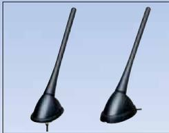
Optional: AN-70DAB (drill mount) / AN-75DAB\* (surface mount) type antenna
