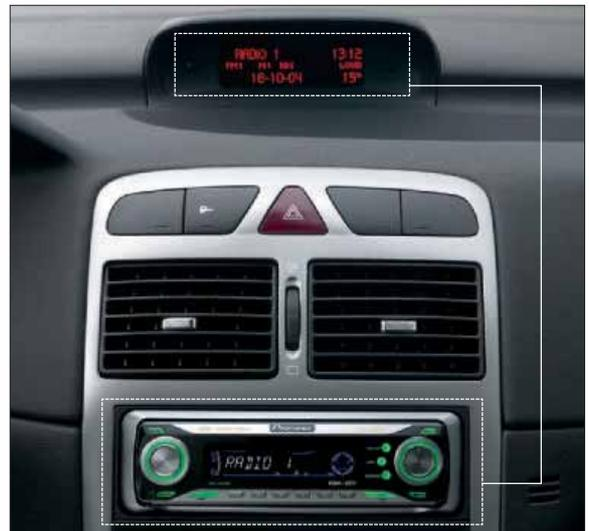
Connect your Pioneer CD tuner\*\* to your car's existing digital display, thanks to the sub-display output feature, and get basic tuner information – such as frequency and track numbers – via an optional interface through the IP-Bus connection.\*
