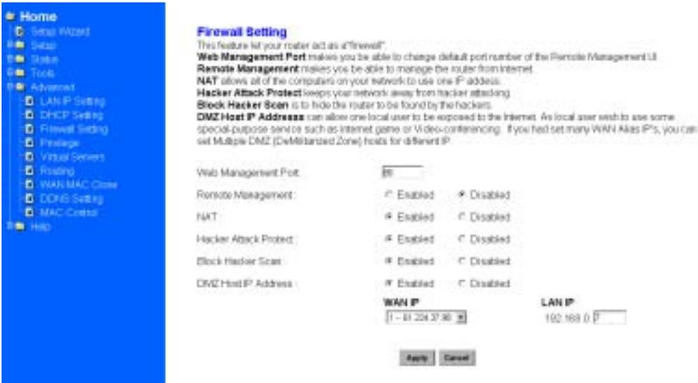
Figure 6-4: Firewall Setting menu with DMZ enabled
