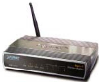
The WRT-410A is a broadband router integrated with an 802.11g Access Point. With the innovative Super G technology enhanced, the maximum data rate of WRT-410A is 108Mbps when working with Super G supported wireless stations. The WRT-410A is also backward compatible and interoperable with IEEE 802.11b compliant wireless devices.
