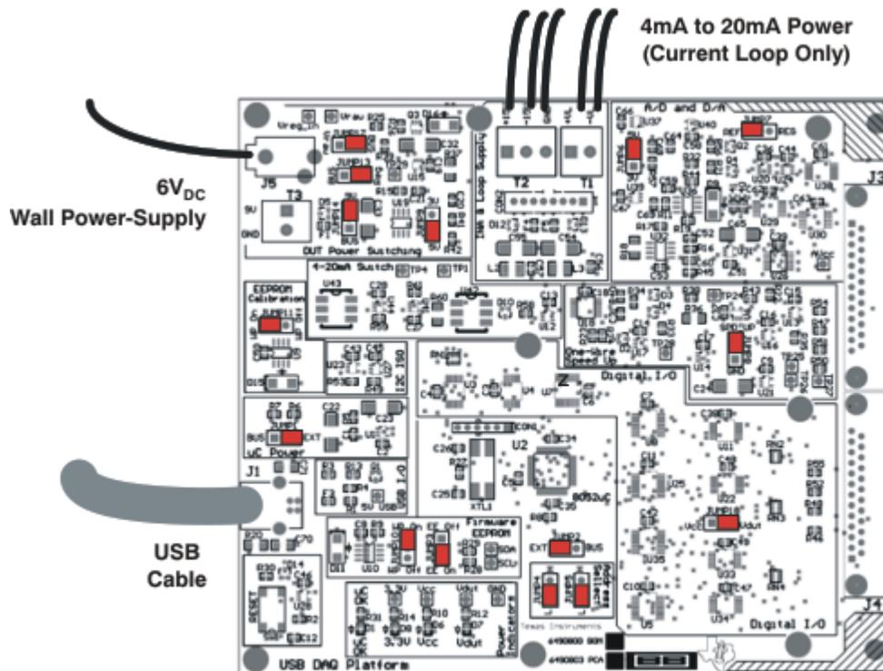
Figure 15. Default Jumper Settings (USB-DAQ-Platform)
