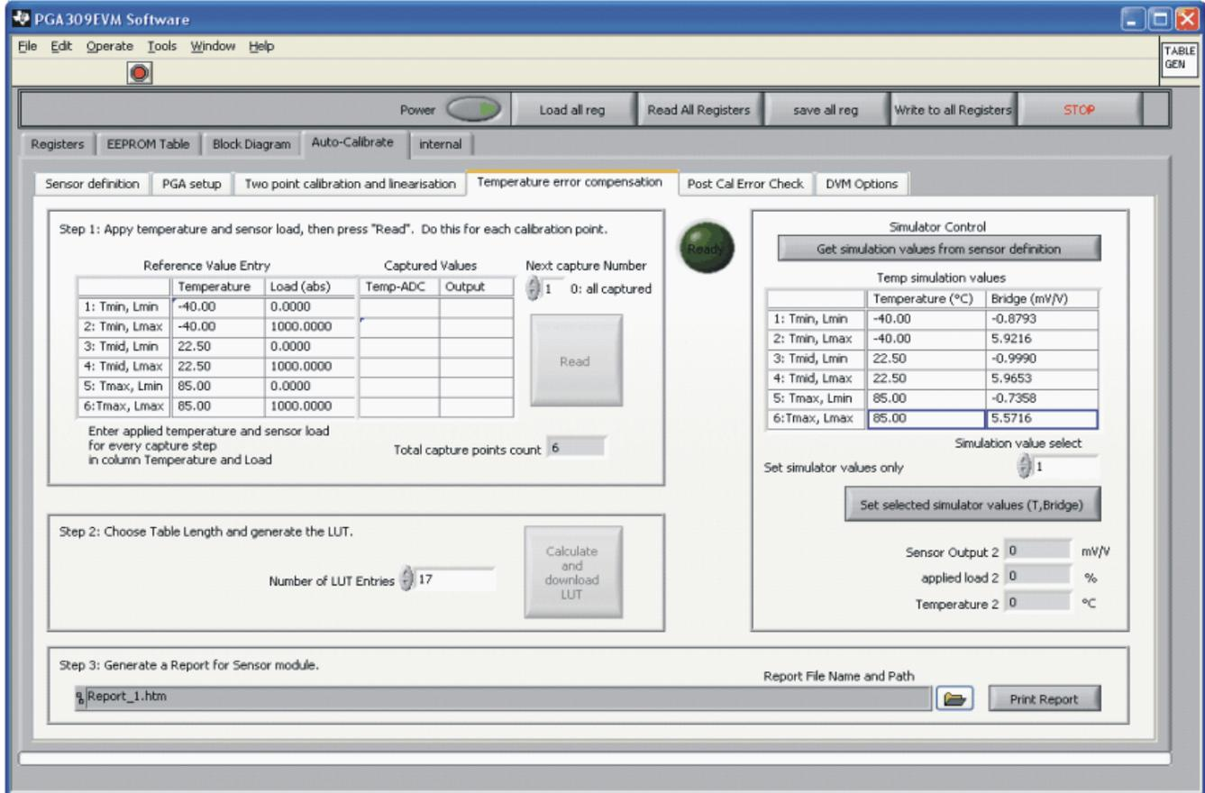
Figure 23. PGA309EVM-USB Software: Auto Calibrate Tab—Temperature Error Compensation
