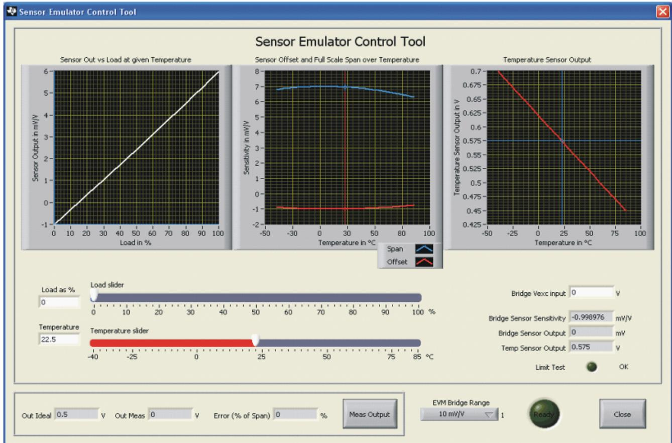
**Figure 20. PGA309EVM-USB Software: Sensor Emulator Control Panel Tool**
