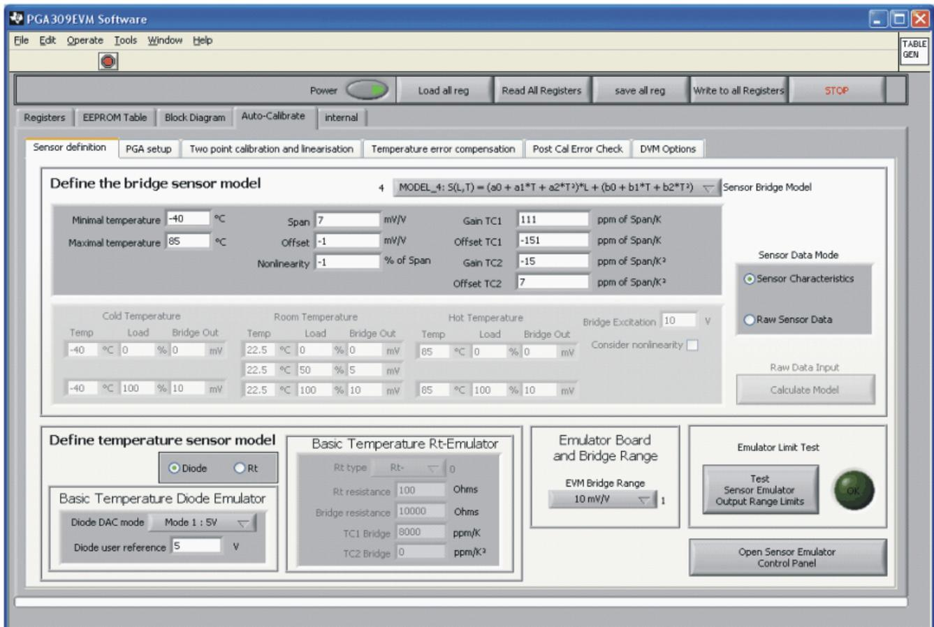
Figure 19. PGA309EVM-USB Software: Auto Calibrate Tab—Sensor Definition
