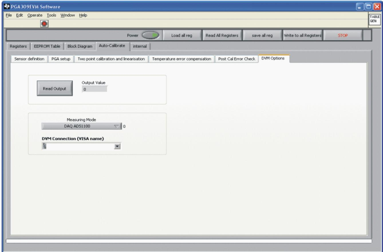
Figure 25. PGA309EVM-USB Software: Auto Calibrate Tab—DMM Options
