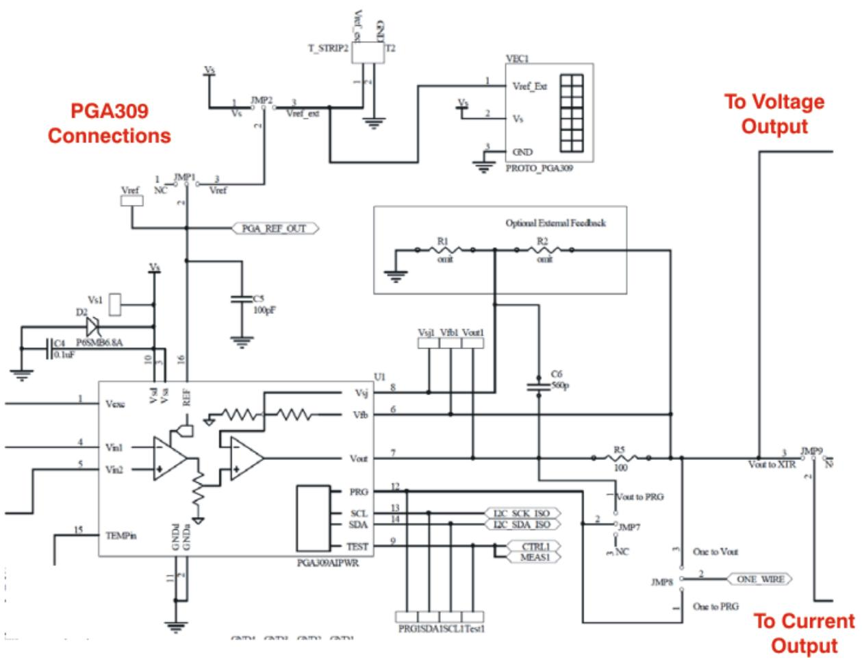
Figure 5. PGA309\_Test\_Board Schematic: Power, Reference, and Digital Connections
