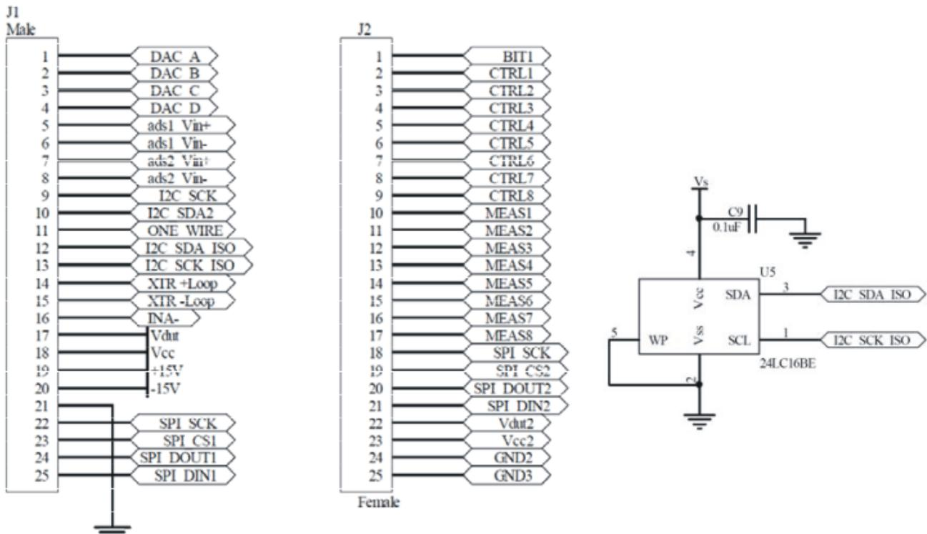
Figure 8. PGA309\_Test\_Board Connections to USB-DAQ-Platform and EEPROM
