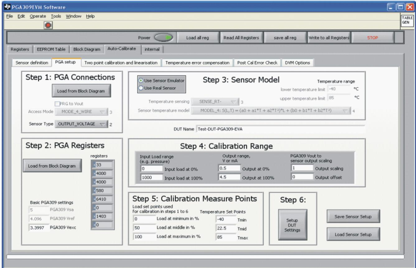
**Figure 21. PGA309EVM-USB Software: Auto Calibrate Tab—PGA Setup**
