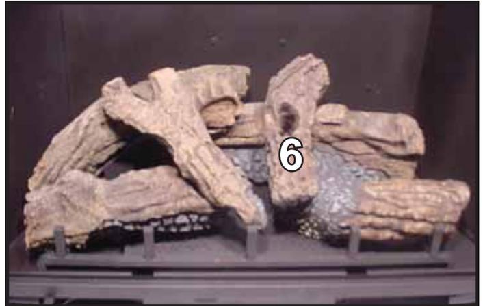
**LOG #6 (SRV327-705):** Rest log #6 in the smooth area just to the left of the knothole in log #1 and on log #3. The front edge of log #1 should be at the top of the hole when looking through the hole in log #6.
