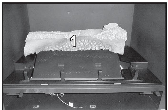
**LOG #1 (SRV349-701):** Place log #1 in the back of the insert. Locate the legs of the log outside the 3/8" tabs to either side of the burner. Pull the log forward until the log is stopped by the back edge of the burner.
