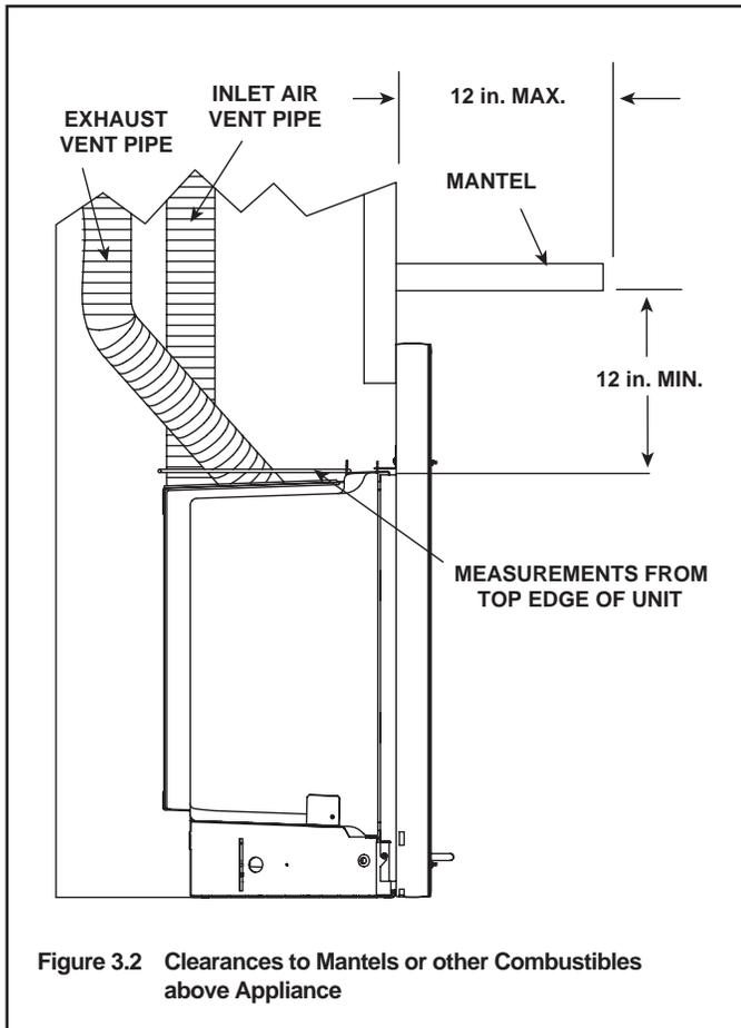
Figure 3.2 Clearances to Mantels or other Combustibles above Appliance
