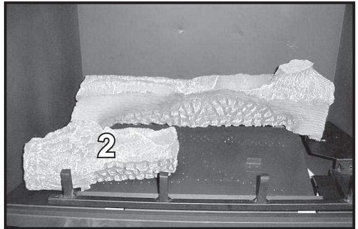
**LOG #2 (SRV349-702):** Position log #2 by locating its slot over the tab on the front left of the burner. The slot of the left side of log #2 fits over the bar grate. Push the left side back so it rests against the step.
