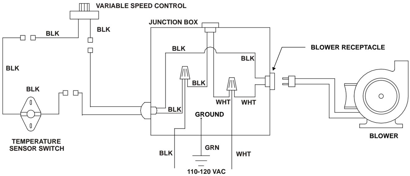
NOTE: IF ANY OF THE ORIGINAL WIRE AS SUPPLIED WITH THE APPLIANCE MUST BE REPLACED, IT MUST BE REPLACED WITH TYPE 105° C RATED WIRE.
