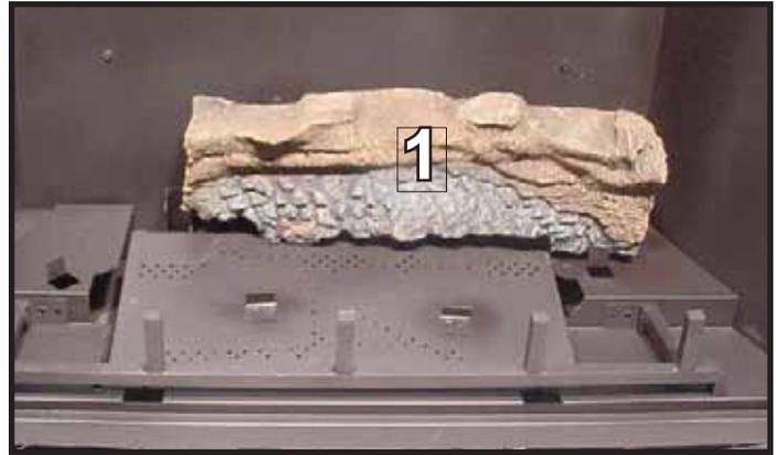
**LOG #1 (SRV339-701):** Place log #1 in the back on the insert. Locate the left end of the log over the center of the pilot and the back side of the left end flush with the back of the pilot bracket. Pull the right end of the log forward until it touches the tab in the base pan.
