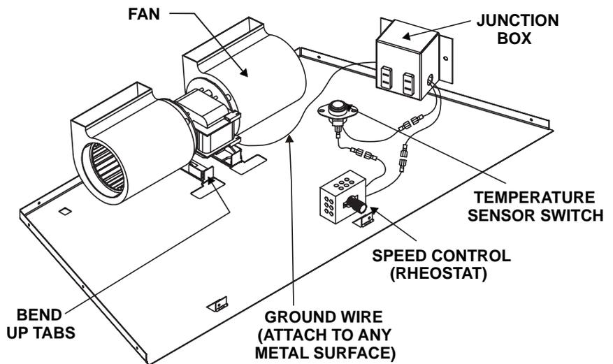
Figure 9.4 Fan/Rheostat Wire Diagram
