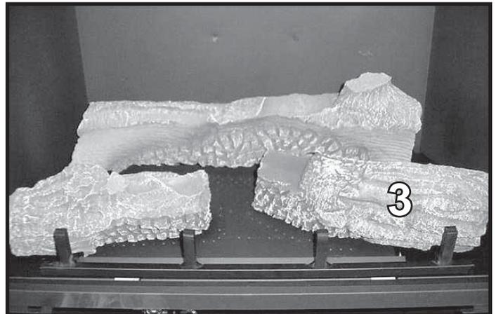
**LOG #3 (SRV327-703):** Position log #3 by locating its slot over the tab on the right front of the burner. The slot on the right side of log #3 fits over the bar grate.
