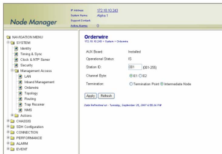
Figure 22. Configuring the Engineering Orderwire (EOW) Function
