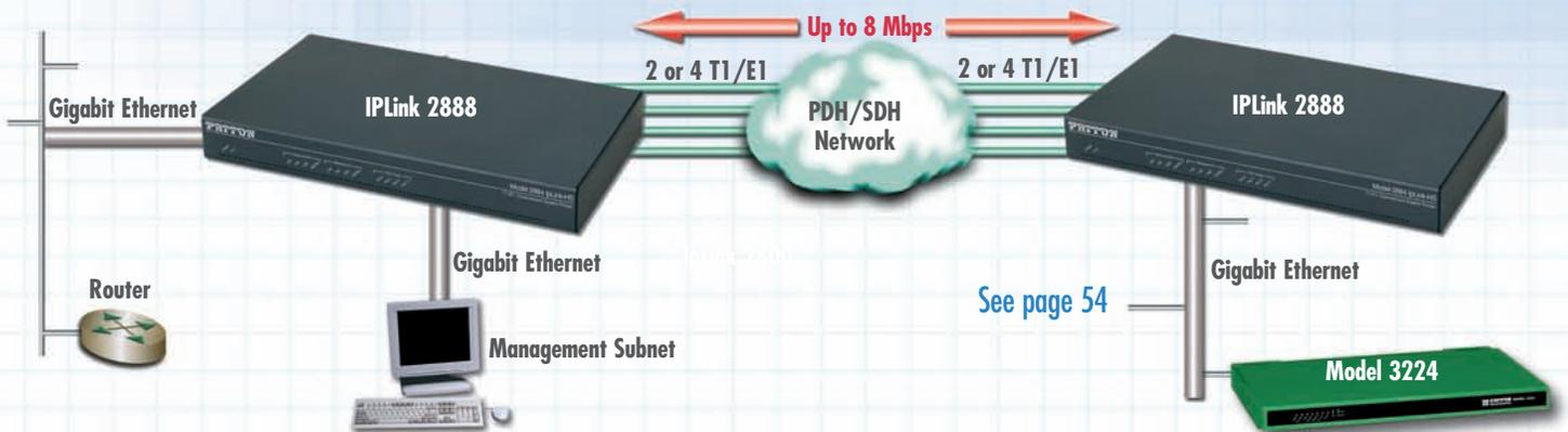
The Model 2888 provides point-to-point high-bandwidth Ethernet/IP connectivity over TDM-based T1/E1 circuits.
