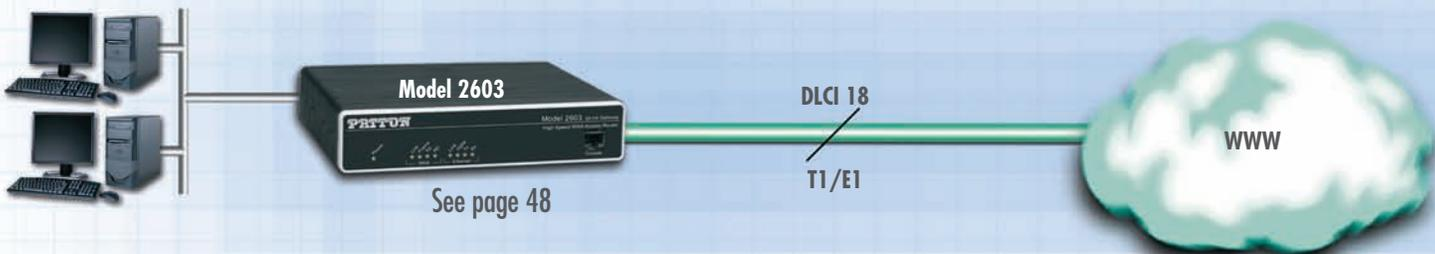
**The Model 2603 T1/E1 Router** provides basic IP access across T1/E1 lines.
