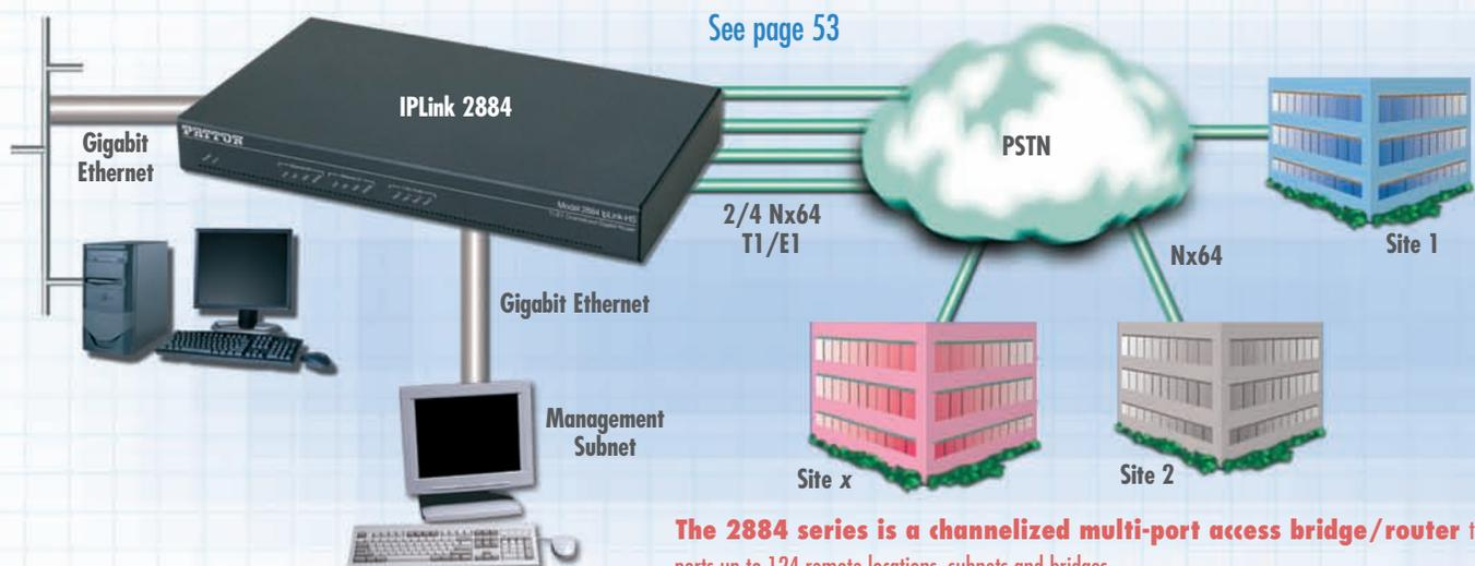
The 2884 series is a channelized multi-port access bridge/router that supports up to 124 remote locations, subnets and bridges.
