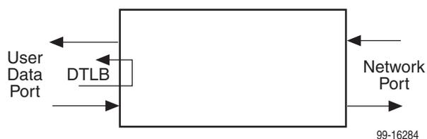
An attached device or test equipment must generate the data to be looped back, and the Port (DTE) Initiated Loopback option must be enabled. Refer to [Configuring the CSU/DSU's Data Port Physical Interface](#) in Chapter 4, *Configuration Options*.
