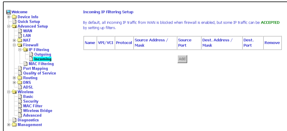
Figure 5-18. IP Filtering – Incoming Filter Setup Page
