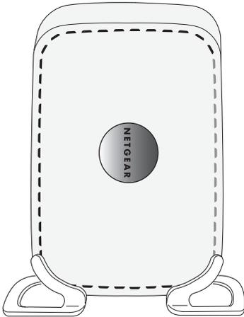
**Figure 4-1: Vertical orientation required on metallic surfaces**
