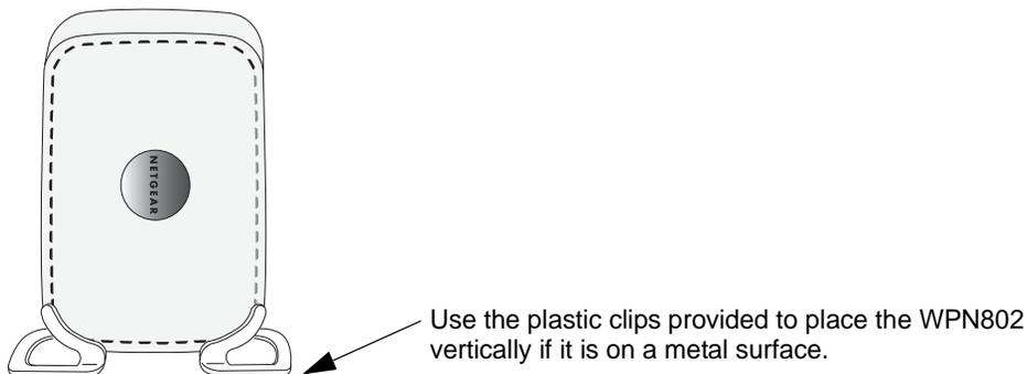
**Figure 3-5: WPN802 placed in a vertical orientation**
