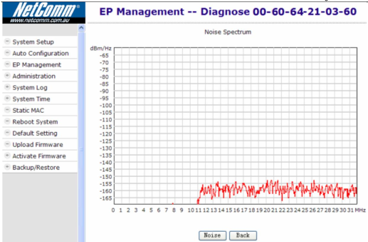
Connect only one EP to Master, with 30dB attenuator add-on. Here's the 'Noise Test' result of the connected EP,
