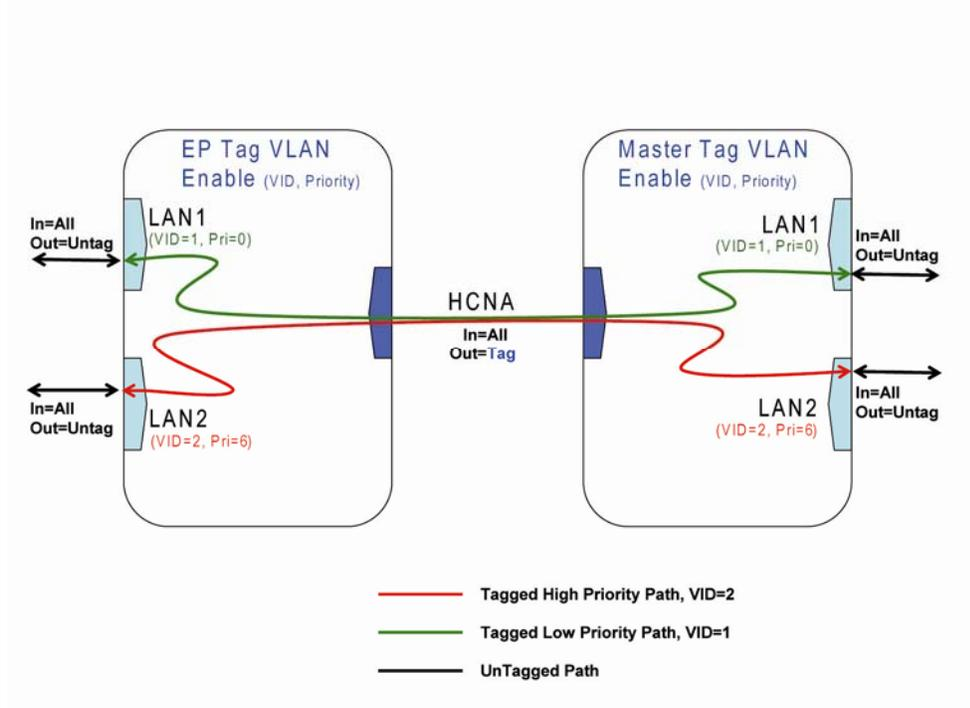
Second example, enable Tag VLAN in EP only, and keep Master Tag VLAN disabled as default, as seen in the following packet path diagram.
