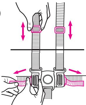
Use slide adjuster at shoulder and waist for tighter adjustment. Repeat on other side.
