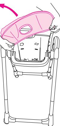
Remove the top of the seat pad from the backrest.
