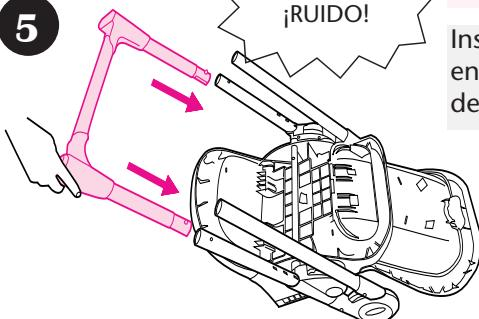
Insert "U" tube into the front leg tubes.
