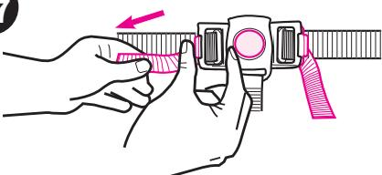
Use slide adjuster at waist for tighter adjustment.
