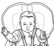
The harness straps must go into the slot that is even with or slightly above the shoulders. Avoid twisting straps.
