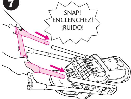
Insert other "U" tube into the rear tubes until they snap into place.
