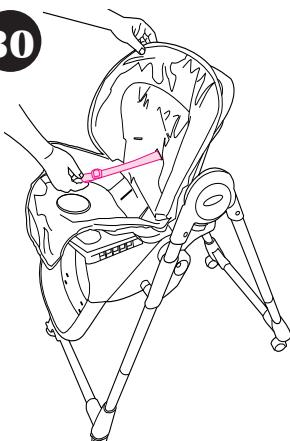
When changing harness strap slots, MAKE SURE harness straps are going through same slots in seat pad and seat back.
