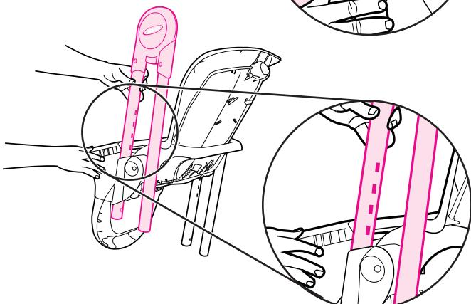
Insert slotted leg post through the frame of the seat, with logo facing out. Repeat with other leg.
