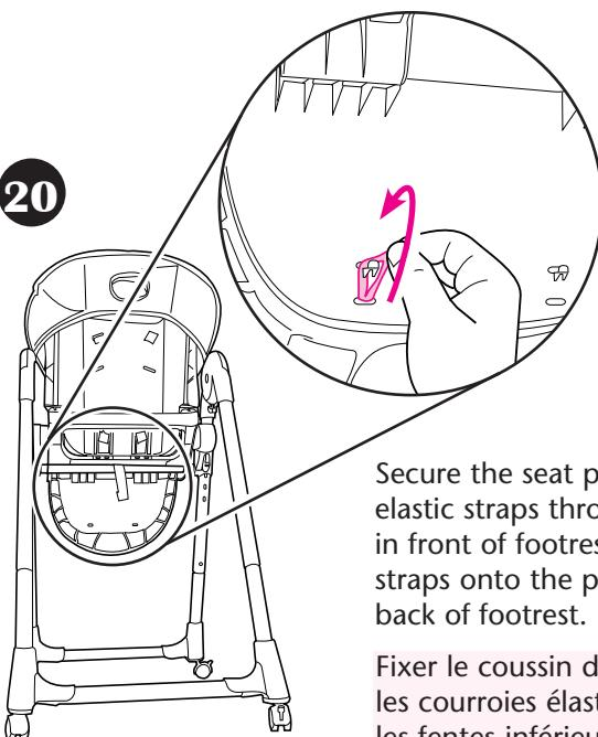
Secure the seat pad by inserting elastic straps through bottom slots in front of footrest, hooking elastic straps onto the plastic hooks on back of footrest.
