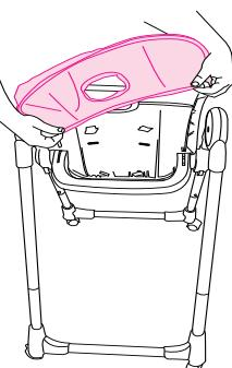
Wrap the top of the seat pad over backrest. Position opening over recline button.
